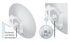
Attach the horizontal slot of the Support Arm to the Upper Pole Bracket using a Hex Head Bolt, Lock Washer, and Flat Washer.
