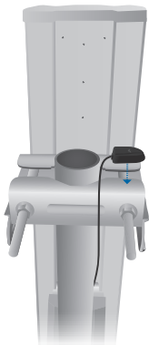
Placement on a Sector Antenna
