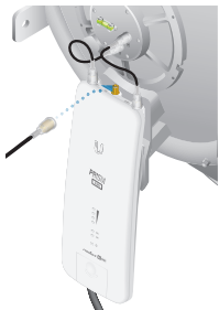
Connecting the GPS Antenna
