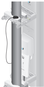
Placement on a Sector Antenna
