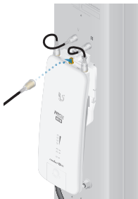
Connecting the GPS Antenna
