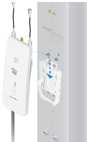
Mounting on a Sector Antenna
