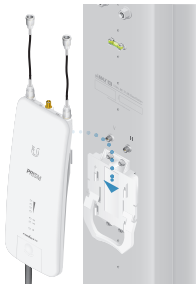
Mounting on a Sector Antenna
