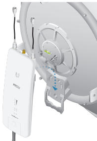
Mounting on a RocketDish
