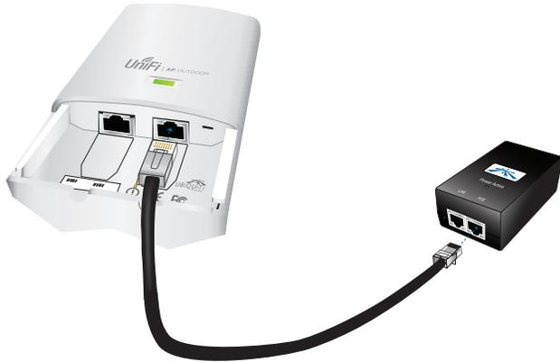
2. Connect an Ethernet cable from your LAN to the Ethernet port labeled **LAN** on the *PoE Adapter*.
