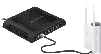
TOUGHSwitch PRO Power Connection Diagram
