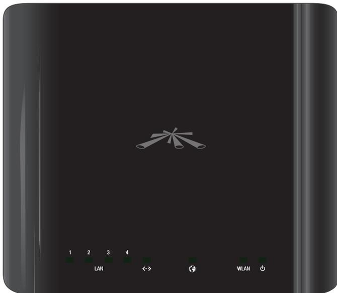
**1-4 LAN** **LAN LEDs (1-4)** Displays the status of the wired connections to Ethernet ports 1-4. Solid green indicates a good connection. Flashing indicates activity on the specific port.
