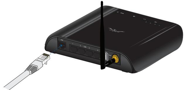
6. Connect the Ethernet connector on the power adapter to your broadband modem. Connect another Ethernet cable from your computer to a LAN port (1, 2, 3, or 4) on the AirRouter HP.
