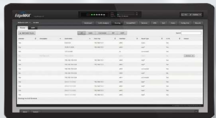
The Routing > Routes screen displays static, connected, RIP, and/or OSPF routes. You can add static routes on this screen.
