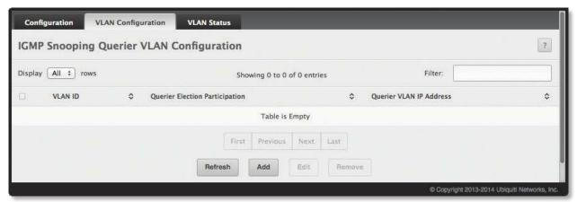
IGMP Snooping Querier VLAN Configuration
