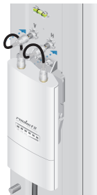
Connecting to a Sector Antenna
