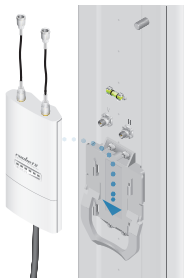
Mounting on a Sector Antenna
