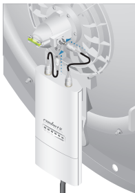
Connecting to a Dish Antenna
