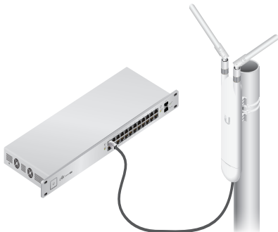
Connected to UniFi Switch, model US-24-250W
