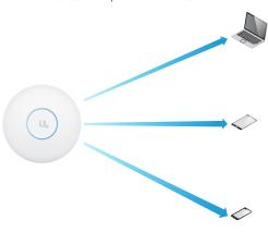
MU-MIMO with 2x2 and 1x1 clients: The UniFi SHD AP communicates with one 2x2 client and two 1x1 clients at a time.
