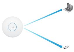
MU-MIMO with 3x3 and 1x1 clients: The UniFi SHD AP communicates with one 3x3 client and one 1x1 client at a time.
