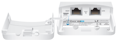
Removing the Tether from the Radio
