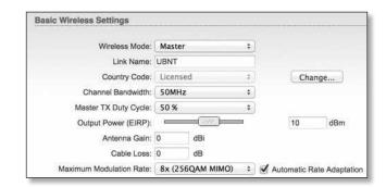
**Wireless Mode** By default, the Wireless Mode is *Slave*. You must configure one AF-5X as **Master** because each PtP link must have one *Master*.
