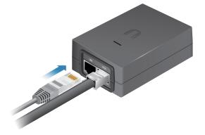
5. Connect the *Power Cord* to the power port on the *airFiber PoE Adapter*. Connect the other end of the *Power Cord* to a power source.
