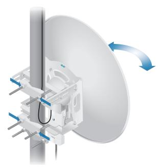
b. Loosen the six elevation bolts, and use the hex nut on the elevation rod to adjust the elevation.
