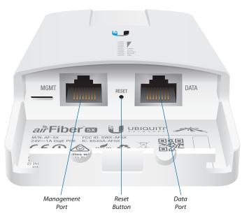
**Management Port** 10/100 Mbps, secured Ethernet port for configuration. *In-Band Management* is enabled by default in the airFiber Configuration Interface. When *In-Band Management* is disabled, the *MGMT* port is the only port that can monitor, configure, and/or update firmware.
