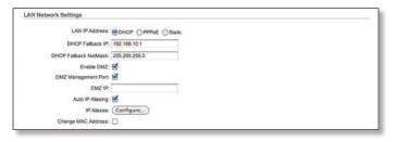
**Enable DMZ** The Demilitarized Zone (DMZ) can be enabled and used so that services such as Web Servers, Proxy Servers, and E-mail Servers can still serve the local network and are at the same time isolated from it for additional security. DMZ is commonly used with NAT functionality as an alternative to Port Forwarding but DMZ opens all ports of the host network device to the external network.
