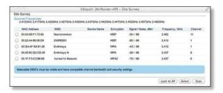
Select the Access Point from the list and click the **Select** button for association. This will automatically enter the name of the Access Point into the SSID field and display the appropriate security options in the *Wireless Security* section at the bottom of the page.
