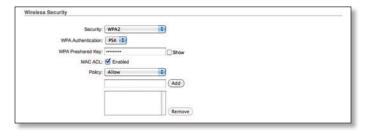
**MAC ACL** (Only applicable in *Access Point* and *Access Point WDS* mode) MAC Access Control List (ACL) lets you allow or deny clients connectivity to the AirRouter HP.
