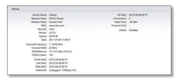
**Device Name** Displays the customizable name (ID) of the AirRouter HP. The Device Name (Host Name) is displayed in registration screens and discovery tools.
