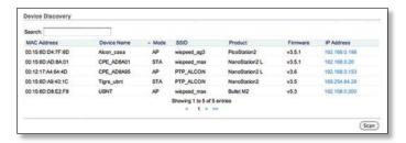
**Device Discovery** Shows device MAC Address, Device Name, Wireless Mode, SSID, Product type, Firmware version and IP Address. To access a device configuration through his Web GUI, click the device's IP Address.
