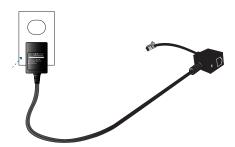
4. Connect an Ethernet cable to the ←→ Main Ethernet port on the power adapter.
