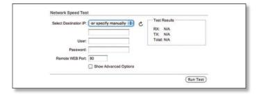
**Select Destination IP** A remote system IP can be selected from the list, which is generated automatically (Select destination IP) or may be specified manually.
