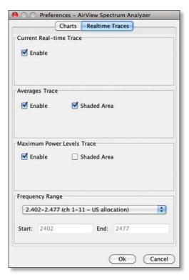
**Current Real-time Trace** When enabled, the real-time trace will be turned on. This is the yellow outline on the *Real-time* chart, which represents real-time power level of each frequency. The refresh speed depends on the FPS.
