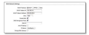
**DHCP Fallback IP** If the AirRouter HP is set to DHCP but is unable to obtain an IP address from a valid DHCP server, it will fall back to the static IP address listed here.
