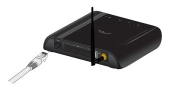
6. Connect the Ethernet connector on the power adapter to your broadband modem. Connect another Ethernet cable from your computer to a LAN port (1, 2, 3, or 4) on the AirRouter HP.
