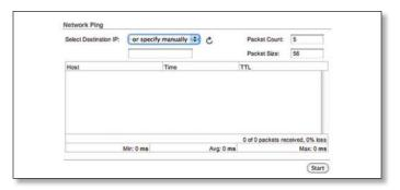
**Select Destination IP** A remote system IP can be selected from the list which is generated automatically or can be specified manually.
