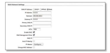
**IP Address** This is the IP address to be represented by the WAN interface which is connected to the external network. This IP address can be used for the routing and device management purposes.
