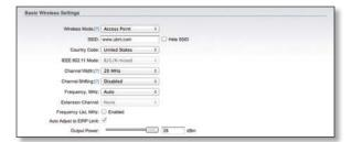
Access Point WDS This is an 802.11 Access Point which allows for Layer 2 bridging with Station WDS devices using the WDS protocol. Access Point WDS is not fully compatible with WPA/WPA2 encryption.
