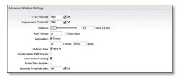
RTS Threshold Determines the packet size of a transmission and, through the use of an access point, helps control traffic flow. The range is 0-2346 bytes, or word "off". The default value is 2346 which means that RTS is disabled.
