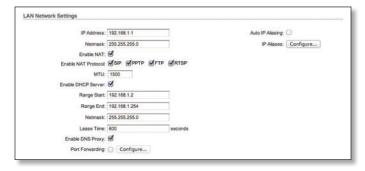
**IP Address** This is the IP address to be represented by the LAN (including WLAN) interface which is connected to the internal network. This IP will be used for the routing of the internal network (it will be the Gateway IP for all the devices connected on the internal network). This IP address is used for the management of the AirRouter HP.
