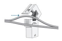
3. Close the opening of the mFi Current Sensor until the latch snaps into place.
